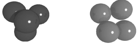
FIGURE 3. Computer generated picture of a very regular tetrahedron ( \sigma_b = 0.02d , left) and a very irregular one ( \sigma_b = 0.22d , right). The spheres are drawn to scale ( d = 2.36\mu\text{m} ).
