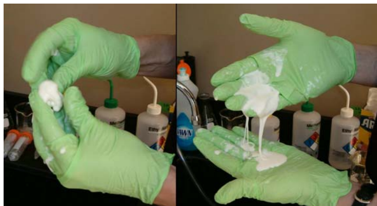
Fig. 1. A corn starch-water mixture can be rolled around in your hand like a ball of soft clay (left), but will then flow like a liquid when you cease rolling it (right).
