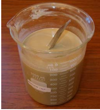
Fig. 2. A metal spatula stays inclined in a mixture of Bentonite and water, suggesting it is an elastic material; yet when stirred by hand with the spatula, it stirs almost as easily as water.
