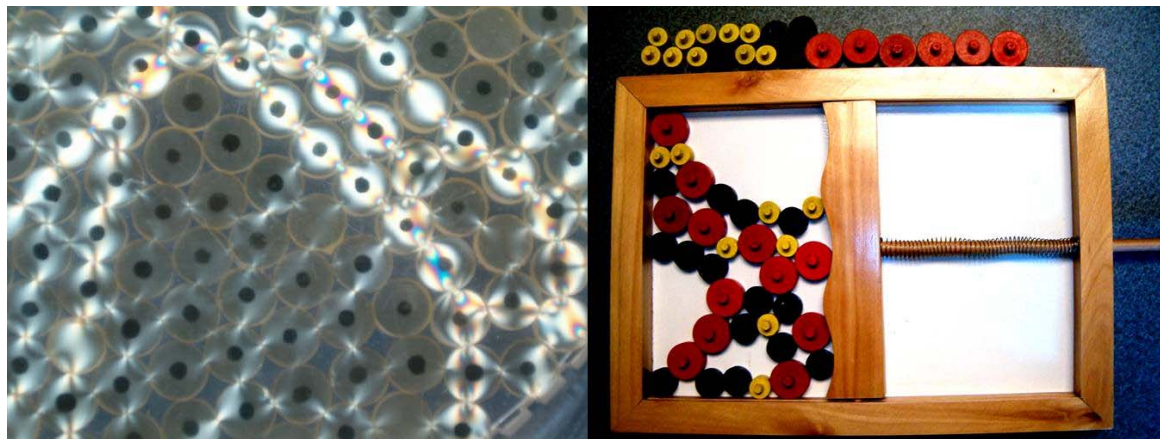
Fig. 3. Left: Photoelastic disks show force chains when viewed between crossed polarizers. Compressed disks are birefringent, and thus appear brighter. The configuration of disks in the old game “Risky” also suggests force chains.
