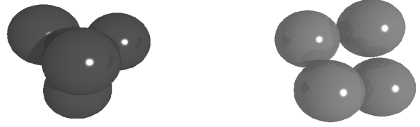
FIGURE 3. Computer generated picture of a very regular tetrahedron ( \sigma_b = 0.02d , left) and a very irregular one ( \sigma_b = 0.22d , right). The spheres are drawn to scale ( d = 2.36\mu\text{m} ).
