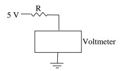
Figure 3. A voltage source connected to a voltmeter through a resistor.
