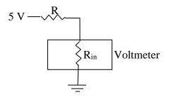
Figure 4. The input resistance of the voltmeter is revealed.
