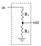
Figure 7. A circuit element known as a voltage divider.
