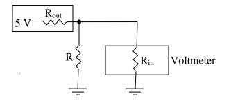
Figure 6. The output resistance of the voltage source is revealed.
