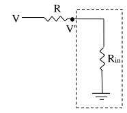
Figure 9. The circuit used to measure R<sub>in</sub>.
