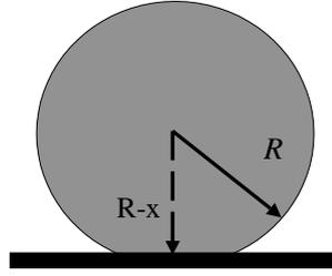
FIG. 1: Diagram of a compressed elastic sphere. The compression distance is  $x$ , so that the centerline radius has been reduced from  $R$  to  $R - x$ .
