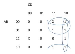
B. Write out any logic equation that implements the K map. You may use as many gates as you like. landfill =  $C\&^D | A\&C | B\&C = C\& (A|B|^D) = C\&(A\&B\&D)$  C. Write out the circuit diagram equivalent to the logic equation.
