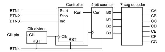
Problem 3. Build a 4-digit decimal stopwatch, with the least-significant digit counting a rate of 1KHz (1ms update rate), and the most-significant digit incrementing once per second (each digit on the seven-segment display will be driven from a separate decimal counter). Use the same controller as was used for Problem 2.
