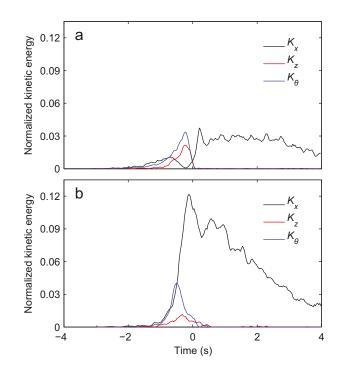
**Fig. 4.** Normalized horizontal, vertical and rotational kinetic energy of an  $\varepsilon = 0.25$  iceberg as it capsizes (a) bottom-out and (b) top-out. The energies are normalized by the total gravitational potential energy released during the capsize event (Burton and others, 2010; MacAyeal and others, 2011) (see also Eqn (20)).
