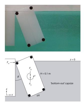
**Fig. 1.** Still-frame and schematic force balance (excluding the drag forces and torque) of the laboratory experiments, where  $F_g$  is the force due to gravity and  $F_b$  and  $\tau$  are the force and torque due to buoyancy. All other variables are described in the text.
