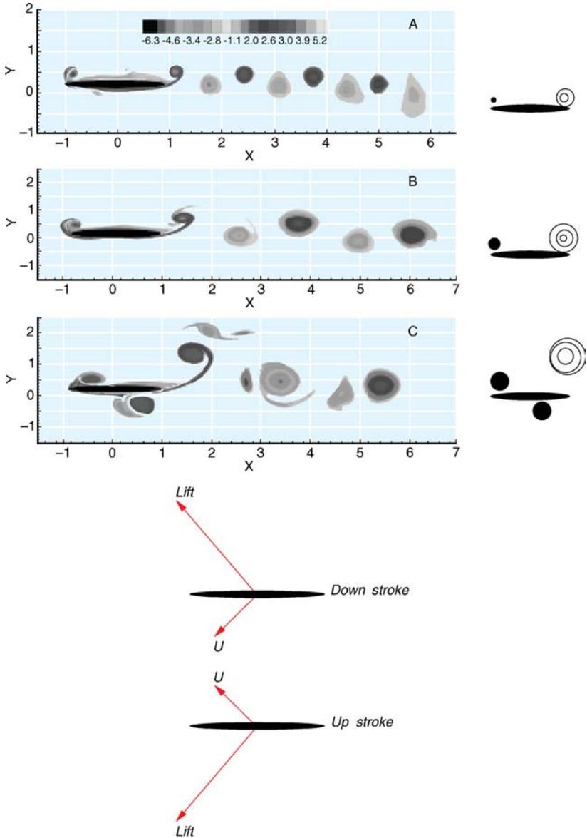
**Figure 5** Forward flight. Top: Vorticity field (reversed von Karman wake) shed by a symmetric flapping wing in forward flight at three frequencies (Wang 2000b). Bottom: The schematic of the thrust generation, which is the forward component of aerodynamic lift.
