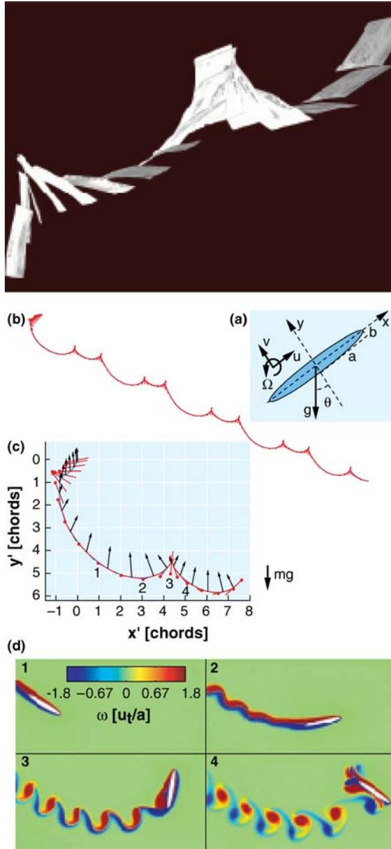
**Figure 9** Falling Paper: Navier-Stokes Solutions, Model of Fluid Forces, and Center of Mass Elevation. Top: Falling paper filmed at 300 fps under windless conditions. Bottom: The Navier-Stokes solution of a tumbling ellipse. (a) Coordinate system, (b) trajectory of the chord (in red) in the first five periods released from rest, (c) instantaneous fluid forces (black) superposed on the chords (red), and (d) vorticity field at four instants during a full rotation (Pesavento & Wang 2004).
