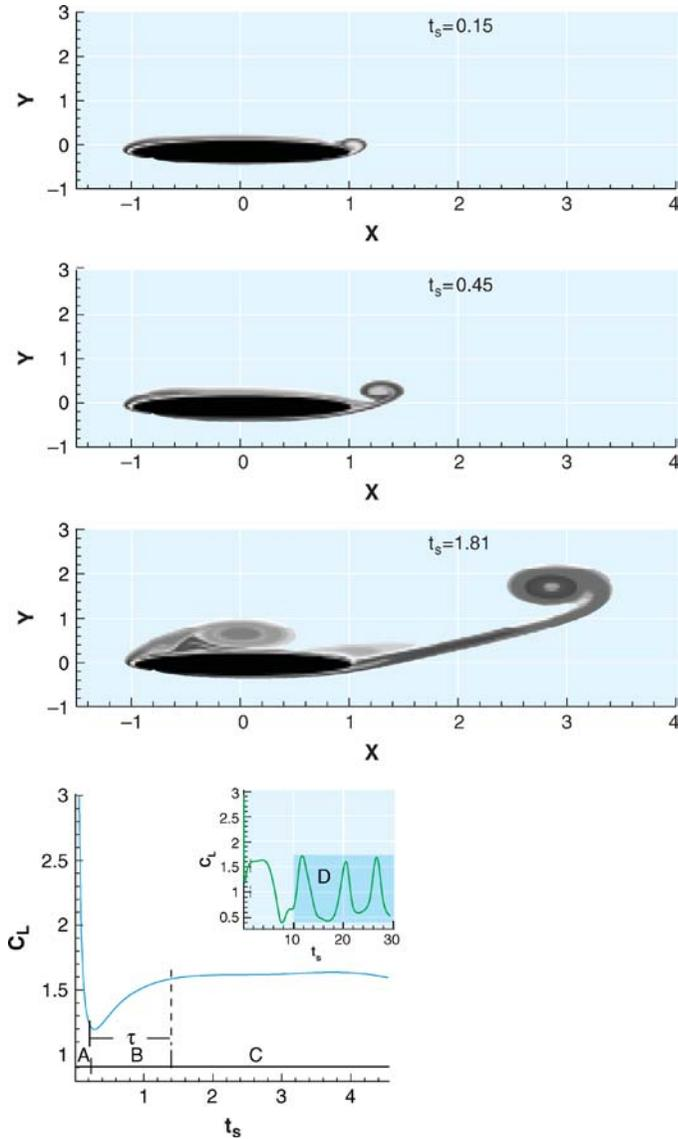
**Figure 3** An impulsively started ellipse of aspect ratio  $1/8$  with an angle of attack  $40^\circ$  and  $Re = 1000$ . Top: Vorticity contour plot. Bottom: Lift coefficient in the dynamic stall regime. Inset: Lift coefficient over a longer time period, up to the von Karman shedding state (Wang 2000b).
