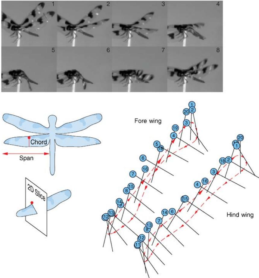
**Figure 1** Top: tethered dragonfly during one wing beat, filmed at 1600 frames per second. The three-dimensional wing kinematics is extracted from two simultaneous views using a mirror. Lower right: the chord positions of fore and hind wing projected onto a two-dimensional slice (*lower left*) (D. Russell & Z. Wang, in preparation).
