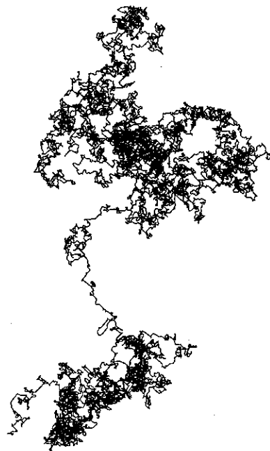
Fig. 1.4. An x, y plot of a two-dimensional random walk of n = 18,050 steps. The computer pen started at the upper left corner of the track and worked its way to the upper right edge of the track. It repeatedly traversed regions that are completely black. It moved, as the crow flies, 196 step lengths. The expected root-mean-square displacement is (2n)^{1/2} = 190 step lengths.
