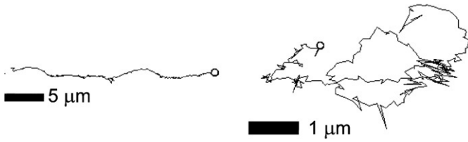
Fig. 14. Example of particle tracks in the laboratory (left) and in the co-moving frame (right). Circles indicate the start of the trajectory. The particle is situated in a shear zone (local shear rate 5 \text{ s}^{-1} ) of a suspension flowing into a square channel with smooth inner walls. The length of the track is \sim 2.3 \text{ s} .
