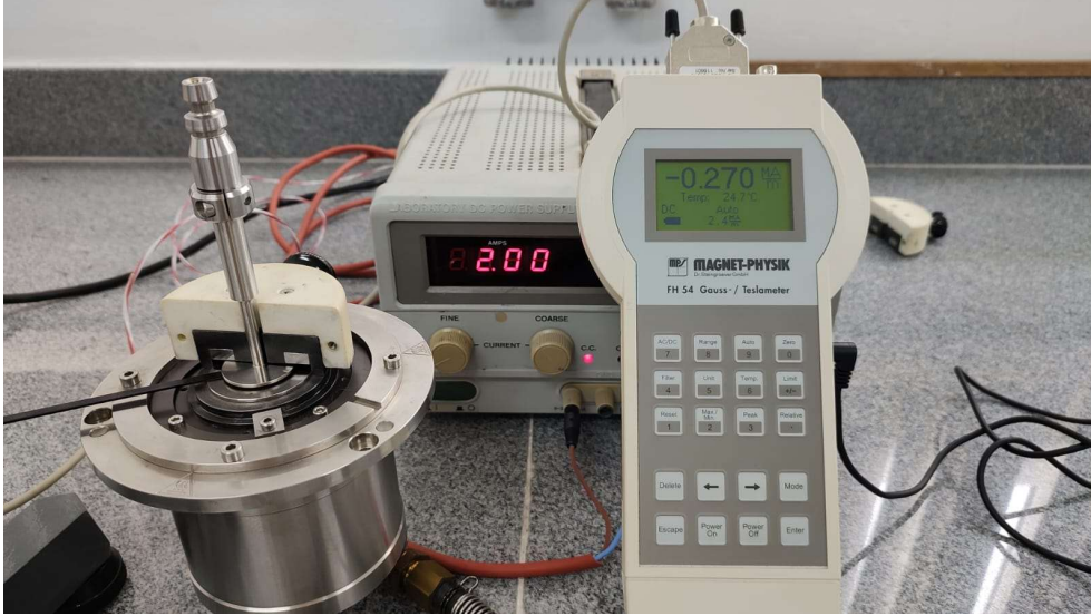
Figure S3 - MRD-180 cell (Anton Paar, 1 st version, 2002) with the Hall effect probe inside the gap between the plates, power supply DC ( I = 2.00 A), and Teslameter “Magnet-Physik” FH-54 showing H = 0.270 MA/m (or 270 kA/m). The gap was empty, in air, and with no MRF sample inside because it is not possible to directly measure the magnetic flux density B with the gap filled with MRF samples, in this MRD cell configuration.
